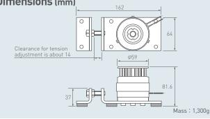
%To be used with Pulley Lock controller
