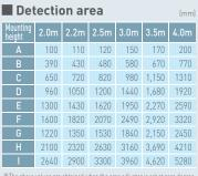
%The above values are obtained when the area adjuster is set at zero degree
