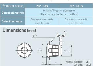
∗To be used with Beam Sensor controller
