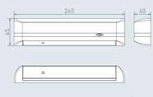
Mass : 260g (MS-N01) 280g (MS-01) Detection area (mm) \*Mounting height shows the height of where sensor is mounted.
