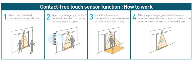
🛕 As contact-free touch sensor by near-infrared reflection method, unlike a mechanical touch switch, it may detect an object at other positions than near touch sticker.
